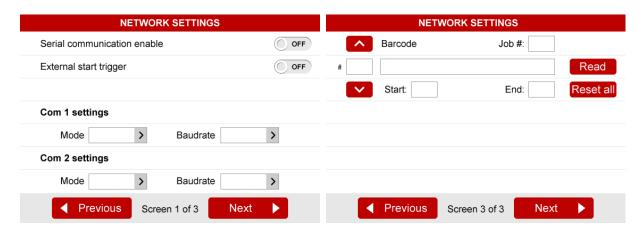
To use serial communication, it has to be enabled by ON/OFF switch in Network settings.
