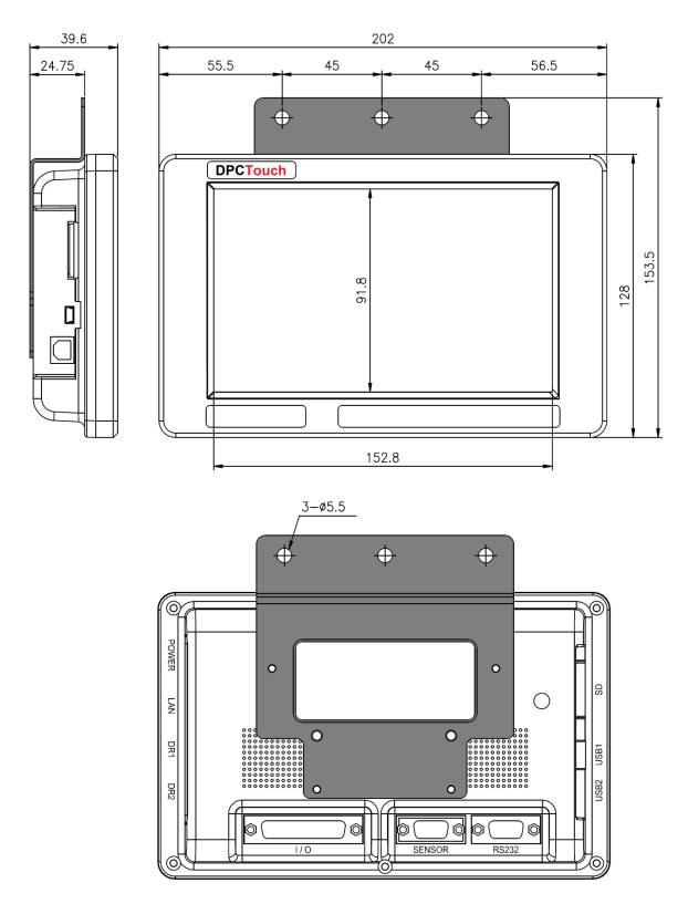
Mounting plate with 4 x M3 screws is delivered with the controller as a standard accessory.
