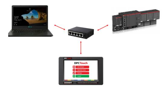
Implementation of Modbus TCP/IP (Ethernet):
