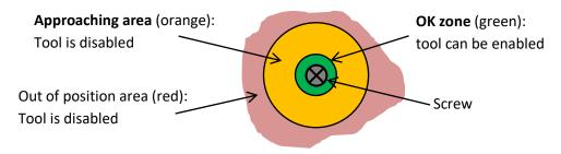
**NOTE:** real shapes of tolerance areas are not circular; they depend on the geometry of the positioning arm being used. To avoid overlapping of tolerance areas of different screws, keep tolerance values as low as possible.
