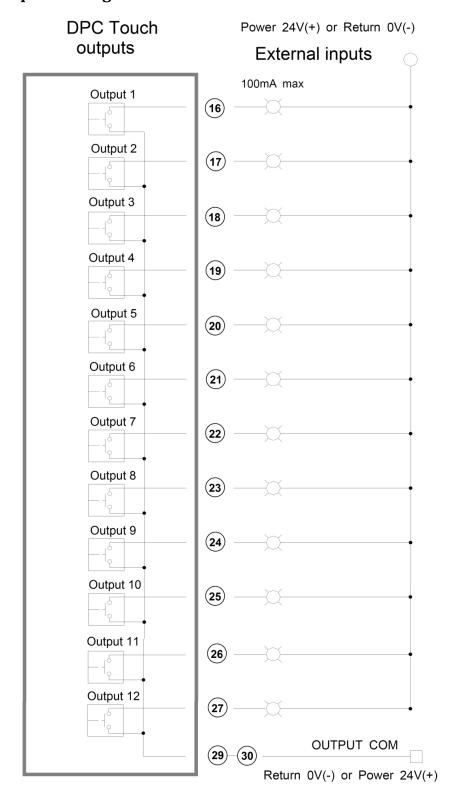
**NOTE:** All outputs are optically isolated. Max current capacity is 100mA per output. Total of 500mA.
