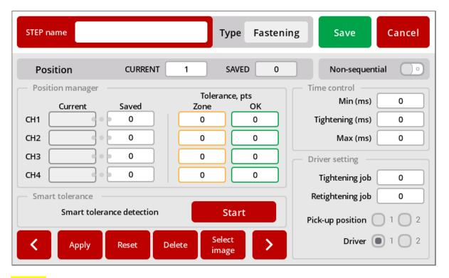
Position Current field displays the number of position being programmed.
